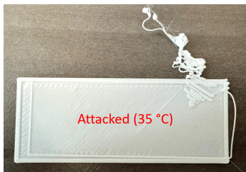
Fig. 14: First Layer Adhesion attack demonstrated at 35°C bed temperature.
