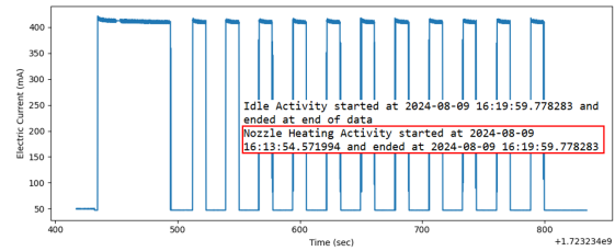
Fig. 10: Nozzle Burning attack signal with 2 recent activity logs.
