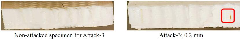
Fig. 17. Attack 3 specimens after bending tests.
