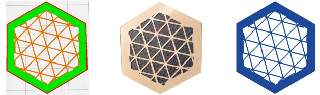
Figure 12: Slicer representation (left), actual printed object (center), and accurate image recovered from FROMEPP dataset (right)
