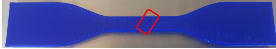
Figure 12: Infill-vertex spacing attack with 0.2 mm magnitude: Image taken after pausing the printing process during one of the attacked layers shows the inverse wedge cavity
